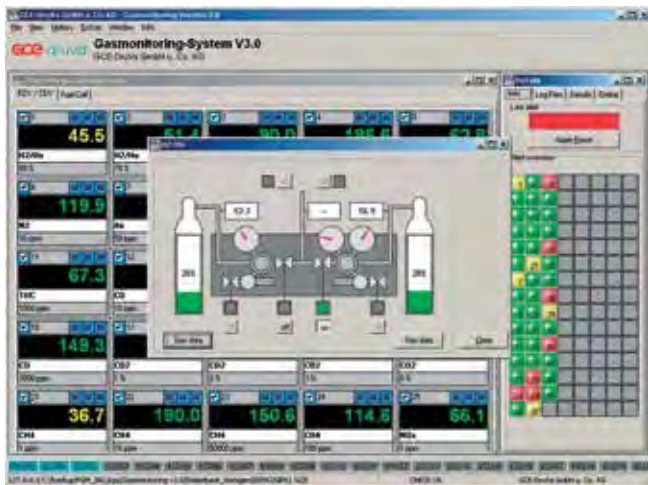
GasCom, stock control and pressure levels, status displays of switching stations, initiating of purge cycles, emergency shut-offs
