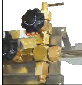
Purge valve with outlet connection mounted on X-block
