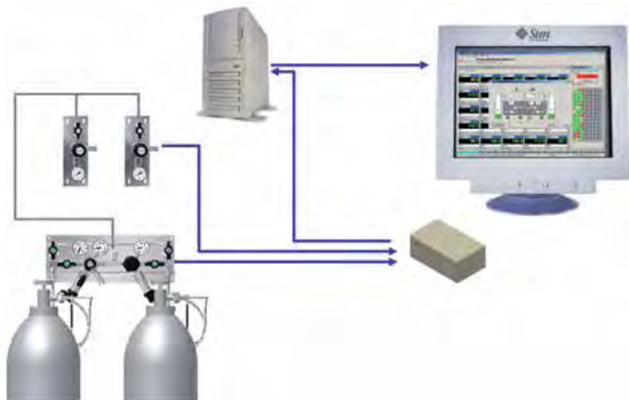
Location-independent monitoring through the Internet or Intranet, remote diagnostics of the central gas supply, archiving of system data, order triggering
