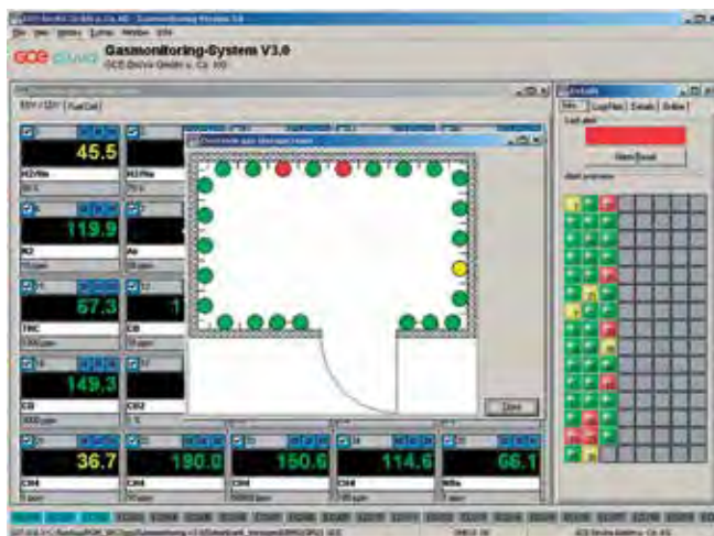
GasCom, graphic display of cylinder pressure with alarm functions and low supply pressure displays
